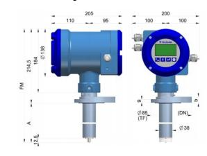
Converter XT5 compact mounting FLOMAT-FX/1/x threaded connection
