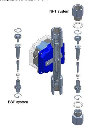
Total length M21 with NPT damping system:  $\frac{1}{4}$ " = 201 mm ;  $\frac{1}{2}$ " = 212 mm ;  $\frac{3}{4}$ " = 222 mm
