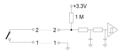
Due to the presence of a filter to avoid the effects of contact bounce, the maximum pulse frequency for the COVOL input is 300 Hz.
