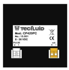
The connection is made in the terminal block marked as mA. The positive terminal of the power supply is connected to the position + and the positive terminal of the load in the position -. The negative terminals of the power supply and the load are connected together. The instrument works in a 2-wire system, that is, the supply and signal line is the same.
