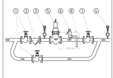
M2F valve should be installed in horizontal pipe and respecting the fluid flow direction must match the arrow on the valve body.
