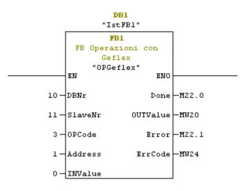
The block requires 5 input parameters and replies with 4 output parameters.
