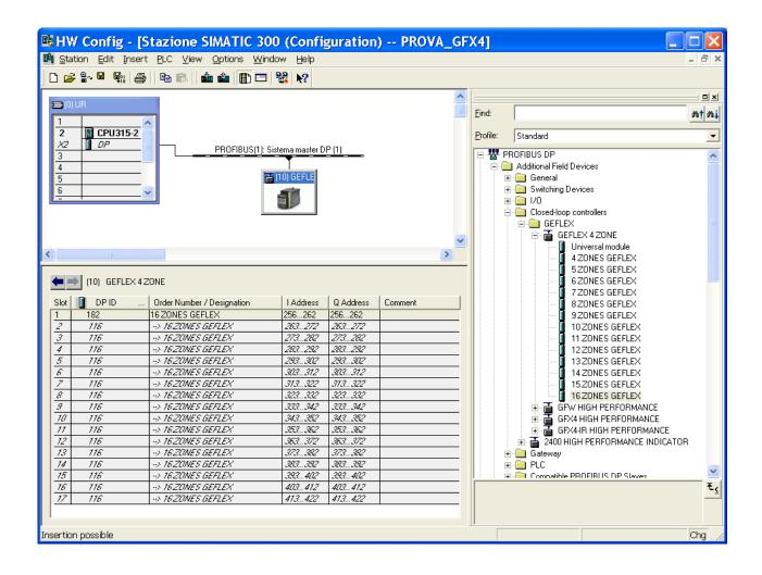
The first 7 bytes in read and the first 7 bytes in write (ID 182) are called "Consistent;" in the figure, they correspond to addresses PEB 256 ... PEB 262; PAB 256 ... PAB 262 and represent the "**Parametric data**" which, controlled via the "OPGEFLEX" Function Block, lets you read or write any variable on the GFX4MODBUS map.
