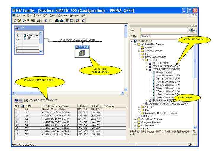
The first 7 I/O bytes (ID 182) are called "Consistent;" in the figure, they correspond to addresses PEB 256 ... PEB 262; PAB 256 ... PAB 262 and represent "Parametric data."
