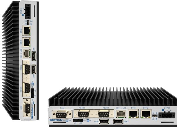
PLC controller contained in electrical panel for high performance solutions with remote monitoring. The performance of the RT VXWorks and the GDnet and EtherCAT realtime field buses make it the heart of the most demanding applications.
