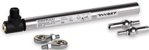
Contactless linear position transducer with patented TWIIST technology for longer life. The lack of contact on the sensitive element creates a completely sealed, robust and compact absolute type linear position sensor.
