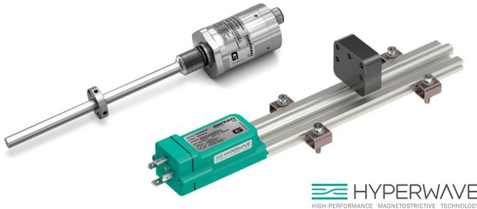
Absolute contactless linear position transducer with HYPERWAVE magnetostrictive technology, with analog output interface. The absence of electrical contacts on the magnetic slider eliminates wear on the moving parts and guarantees a theoretically infinite lifespan. Total protection with ideal use even in difficult environments with high levels of dust and percolating liquid contamination. Excellent linearity, repeatability and resistance to mechanical vibrations and shocks.
