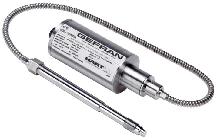
The Gefran "NaK" series of pressure transmitters are state of the art products suitable for use in very high temperature environments. Thanks to well proven Gefran Sodium-Potassium (NaK) filling technology, the average temperature can go up to 538°C (1000°F) while maintaining excellent stability.
