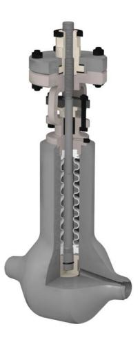
Valves used in the primary heat transport system of nuclear power plants are designed in accordance with ASME Boiler And Pressure Vessel Code, Section III, Subsection NB. They have to answer to three major technical requirements: tightness of sealing system to prevent radioactive fluid leakages to the ambient, construction able to withstand earthquake loads, construction able to pass normally required endurance tests at service condition.
