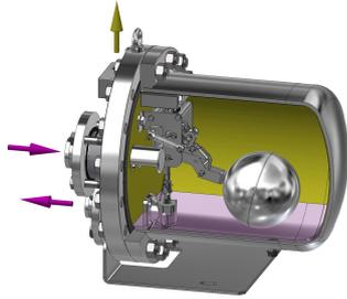
1. In the first instance, the steam intake valve is closed, while the vent valve is open. As condensate flows into the body through the inlet check valve, the PPT14 can operate in a closed loop application, in one of two ways (as a steam trap or pressure operated pump).
