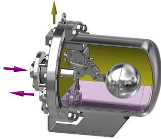
2. If the inlet pressure is greater than the back pressure, the PPT14 works as a steam trap, continuously discharging condensate by differential pressure. At this point the steam intake valve remains closed and the vent valve open.
