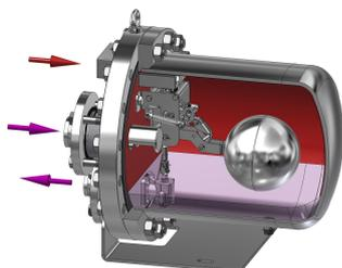
5. The float starts to fall as the condensate level inside the body drops and is discharged to the return system. When the float reaches its lowest position, the snap action mechanism resets.
