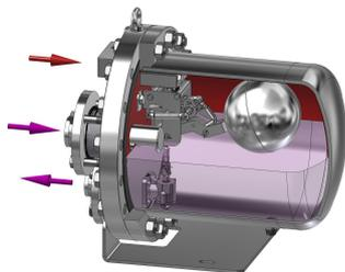
4. If this situation would persist, the condensate would eventually flood the equipment, causing problems. However, by using a PPT14, as the float reaches its highest position, the snap action mechanism actuates, closing the vent valve and opening the steam intake valve. Steam will then replace the necessary positive pressure to pump out the condensate. At this point the PPT14 works as a pressure operated pump.
