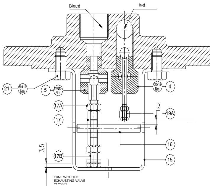
**Adjustment of upper level switch on POP-S and PPO-14 till DN80:**
