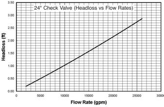
Sample Flow Rate vs Headloss Graphs. Other size charts available upon request. Based on flow testing at Utah State University.
