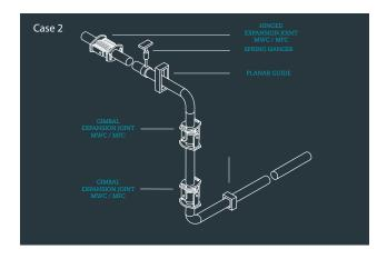
When it is either impossible or undesirable for the horizontal sections of piping to absorb the expansion of the vertical section, a system composed of two Gimbal Expansion Joints plus one Hinged Expansion Joint must be used as shown in the diagram. The use of a Hinged Expansion Joint is justified by the fact that movement in the vertical section only occurs in one plane.
