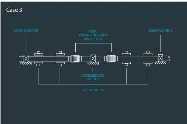
Owing to the size of the straight section of pipe, the Axial EJs are fitted in a way that they are joined together by an intermediate fixed point, thus forming a single unit, similar to an Axial EJ fitted between two main fixed points.
