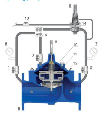
The CSA Model XLC 395/495 is operated by a two ways pilot (5), with pre-set and adjustable set point value, sensing two pressures points in order to maintain a required differential between them.
