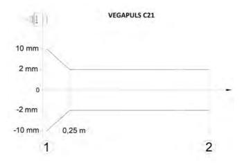
Where for each sensor (1) is the antenna edge and reference plane, and (2) is the recommended measurement range.
