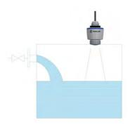
In the case of open tanks with possible sudden level variations or turbulences caused by cyclone suction, it is recommended to mount the sensor inside a protection tube with a length up to the minimum reading level and to provide an aeration orifice of about 5 .... 10 mm diameter (see figure).
