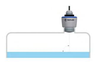
When measuring solid products, the instrument must be aligned in such a way that the radar signal reaches the lowest level of the vessel. In case of a cylindrical silo with conical outlet, the installation is carried out in a position corresponding to one third to one half of the vessel radius (r) (see figure).
