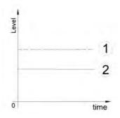
Where (1) shows in dashed line the actual level and in (2) the solid line shows the level indicated by the sensor.
