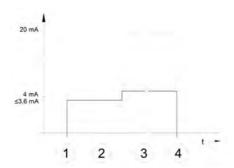
Where: (1)  $U_B$  On, (2) Run-up time, (3) Measured value output and (4)  $U_B$  Off.
