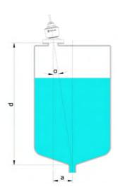
Checking the orientation of the transmitter angle can be done easily with a bubble level. The following table shows the required angle of inclination, which depends on the measuring distance (d) and the distance from the center of the tank to the transmitter (a).
