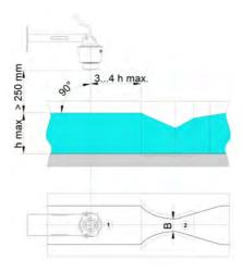
The following figure shows the scheme for the case of application in a rectangular channel. It consists of a spillway gate side view (1) and downstream view (4), which separates upstream (2) and downstream (3).
