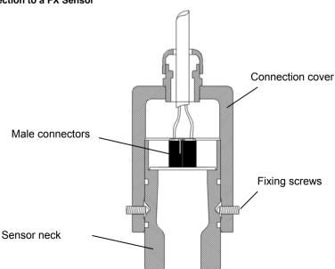
To connect to the sensor, first loosen the cable gland to allow the cable to slide in it.
