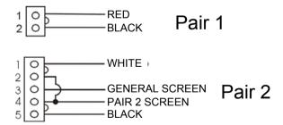
Terminals 2 and 4 of the 5 way connector should be connected together.
