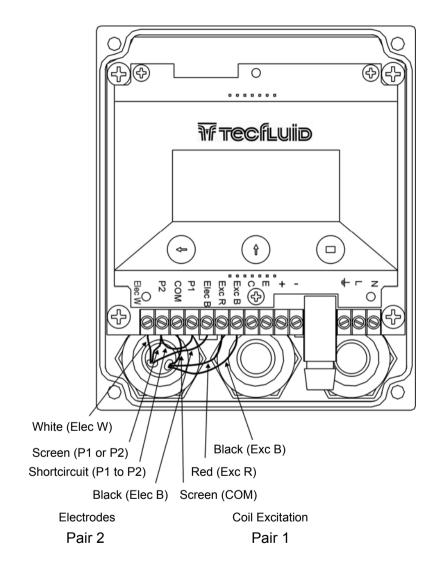
The Pair 1 cables are connected to terminals Exc B, Exc R & COM for the coil excitation. The Pair 2 cables for electrode connection are connected to terminals Elec W, Elec B, P1 & P2. Terminals P1 & P2 must be connected together.
