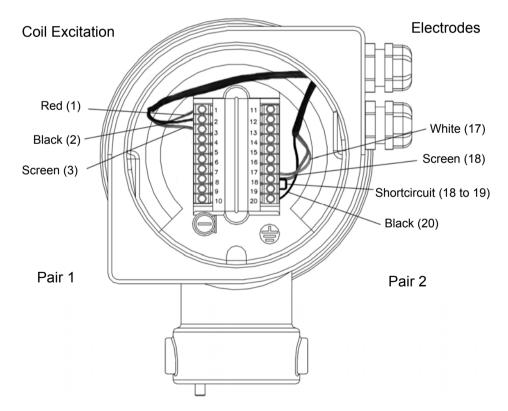
The Pair 1 cables are connected to terminals 1, 2 & 3 for the coil excitation. The Pair 2 cables, for the electrode inputs, are connected to terminals 17, 18, 19 & 20. Terminals 18 & 19 must be short circuited together.
