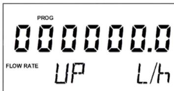
In a CH420P, if during the programming sequence we receive a HART™ command that must be attended, the local programming will not be valid and all the data previously programmed will be lost. The screen will return to the normal working model and the word PROG will light on the screen, indicating this event. To remove the word PROG from the display, press key "Up arrow" or "Left arrow".
