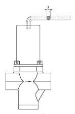
Compressing the spring  $({f anticlockwise})$  increases the outlet pressure
