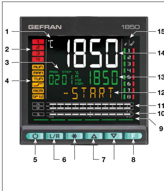
Figure 5 - Description of 1850 display and keys
