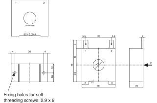
These transformers are used to measure current at 50  $\div$  60Hz from 25A at 600A (rated primary current lp). The special characteristic of these transformers is the high number of turns of the secondary (Is). This produces a very low secondary current, appropriate for an electronic measurement circuit. The secondary current can be read as voltage on a resistor.
