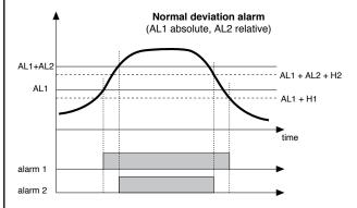
For AL1 direct absolute alarm (max) with negative H 1, A1 t = 0 For AL2 direct relative alarm (max) with negative H2, A2 t = 2
