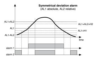
For AL1 direct absolute alarm (max) with negative H1, A1 t = 0 For AL2 symmetrical deviation alarm H2, A 2 t = 6
