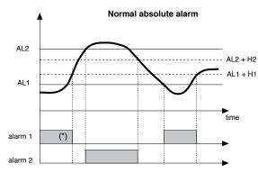
For AL1 inverse absolute alarm (min.) with positive H1. A1 t = 1 (\*) = OFF if disabling on power-on exists For AL2 direct absolute alarm (max) with negative H2, A2 t = 0
