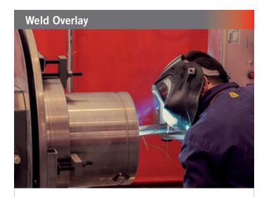
JC Valves provides the best welding technology for any kind of welding needs. Weld Overlay is a welding process, offered on request, where one or more metals with specific characteristics are applied to a base metal to improve desirable properties or to restore the original dimension of the components that significantly enhances the service life of them.
