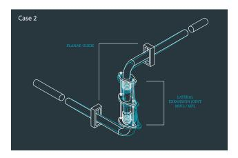
This case shows how an MWL or an MFL Expansion Jont can be used to absorb the thermal Expansion in a Z- shaped section of piping which occurs in three different directions. The fact that this type of Expansion Joint is captable of absorbing lateral movements in more than one direction means that two horizontal pipes can form any angle in that plane.
