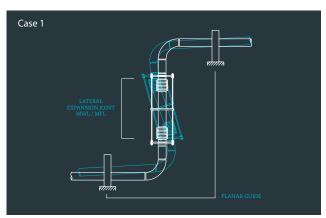
This case illustrates how one MWL or MFL Expansion Joint can be used to absorb the thermal Expansion in a Z-shaped section of piping which only occurs in one plane.
