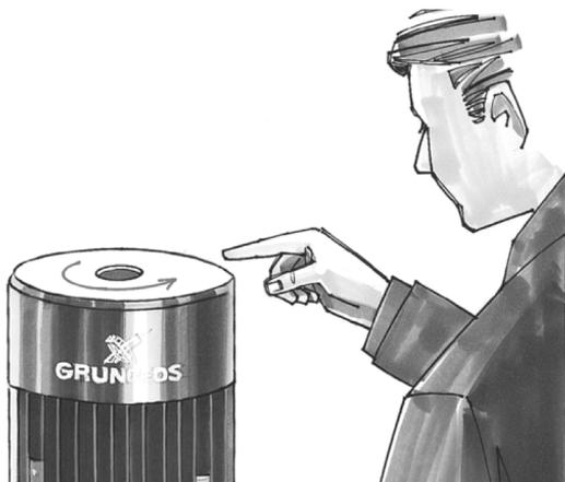
3. See the correct direction of rotation of the pump on the motor fan cover.
